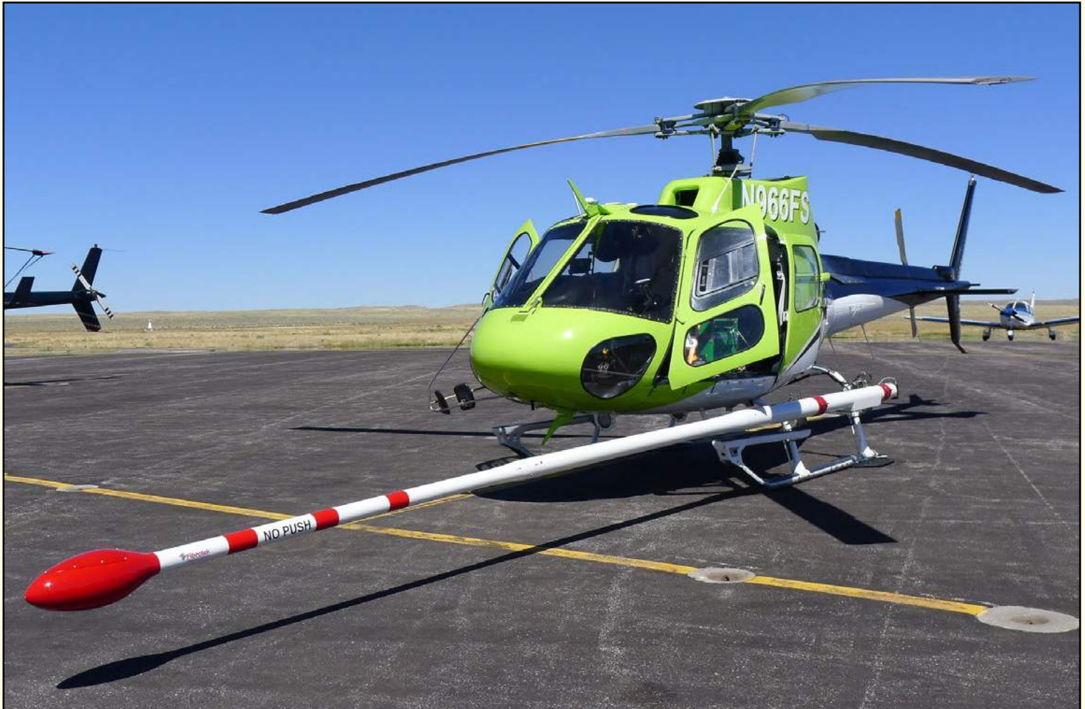
A helicopter equipped with a stinger-mounted magnetometer and gamma-ray spectrometer conducted flights last summer to collect critical mineral survey data. Photo courtesy of WSGS
