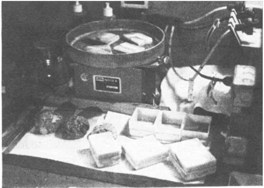
A flat lap machine is simple to operate, but does demand fairly constant attention, with hourly inspections and additions of water.
