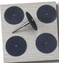
Cutoff wheels are inexpensive and do a great job cutting or shaping steel. You can use them to sharpen tool points, cut piano wire to length, make slots, and sharpen worn drills.
